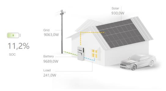
The image below shows the real-time power map of the energy storage system with an EV-charger installed:
