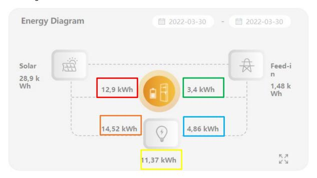
The image below shows the energy flow chart of the energy storage system with an EV-charger installed:
