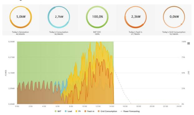
The image below shows the power diagram of the energy storage system with an EV-charger installed:
