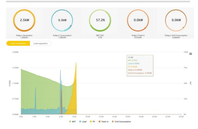
Click on "Load combination" to see the power diagram where the user loads and the EV-charger loads are combined into a total load:
