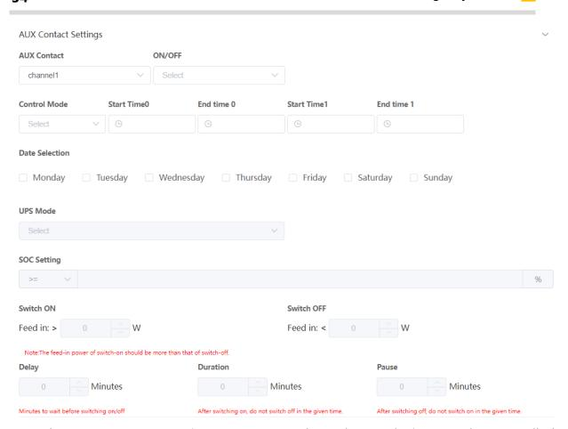
2. Select AUX 1 or AUX 2 in AUX Contact Channel. Two devices can be controlled totally.
