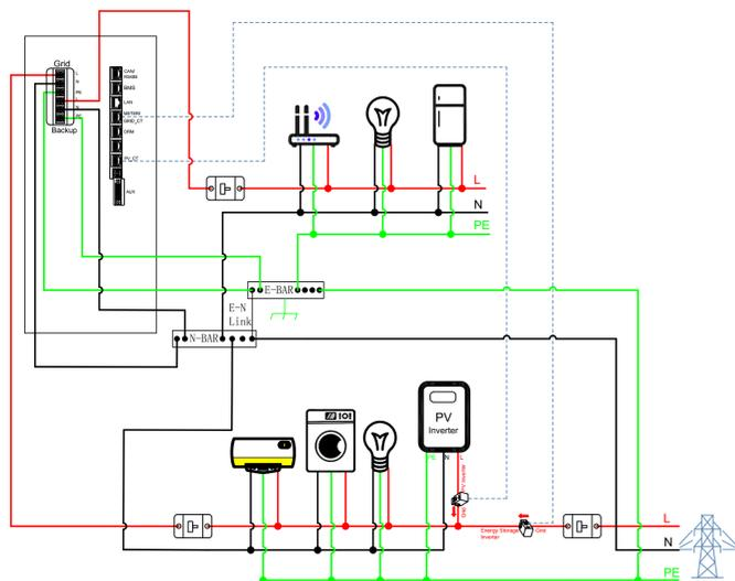
**Step 9** Connect Grid and Backup wire harness, as shown in Figure 2.13.
