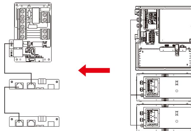
Figure 2.37 Connect the Battery Communication Line
