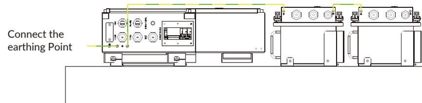
Figure 2.38 Connect the Grounding Harness
