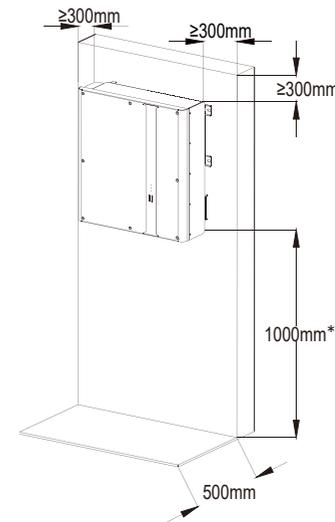
The clearance below is a 'recommendation' only and a minimum of 150 ~ 200 mm off the ground was advisable to protect from submergence.
