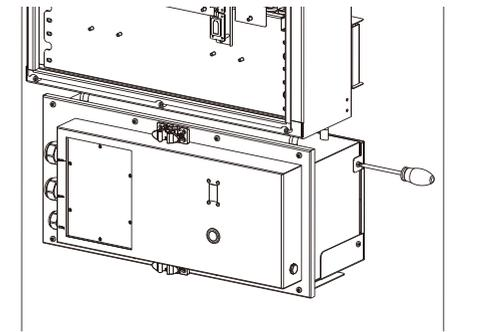
Figure 2.26 Fix the Battery to the Wall Bracket
