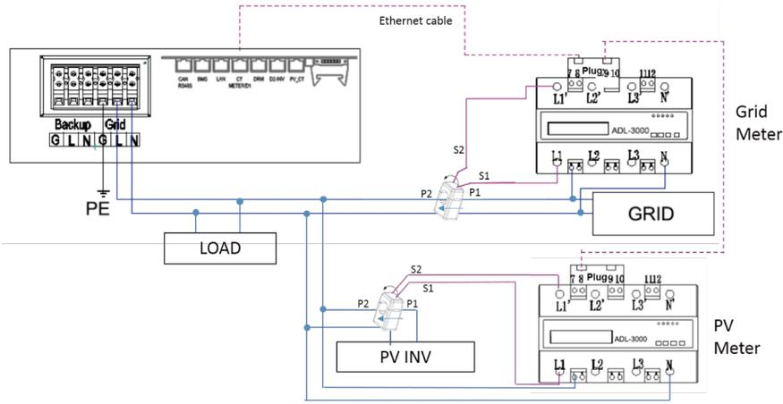
Figure 2.47 ADL-3000 Connection (with CT and Meterplug)
