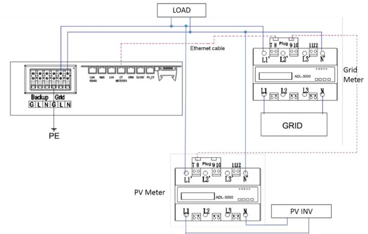
Figure 2.45 ADL-3000 Connection (without CT, with Meterplug)
