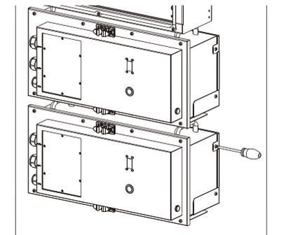
Figure 2.32 Lock the Battery to the Wall Bracket
