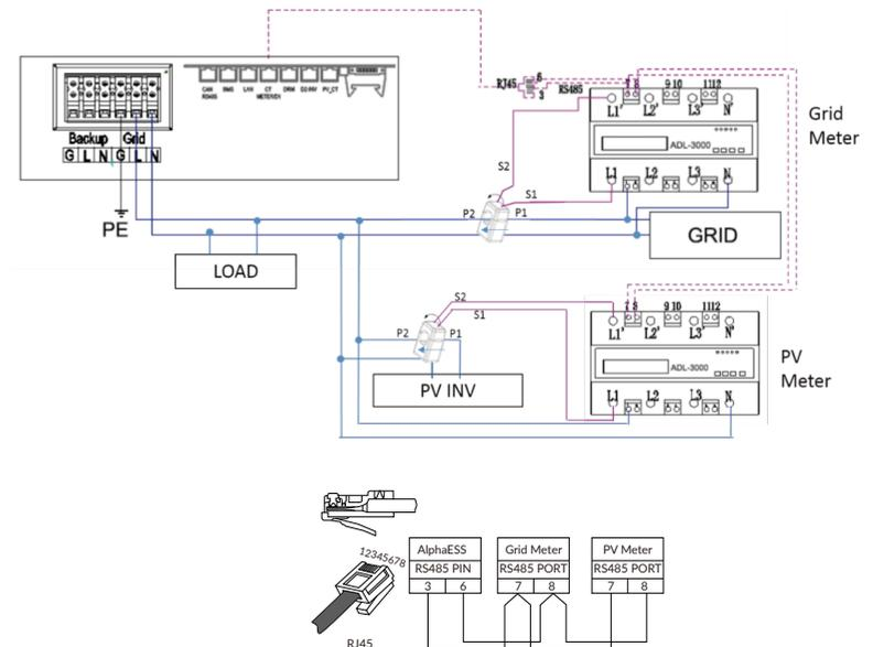
Figure 2.46 ADL-3000 Connection (with CT, without Meterplug)
