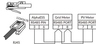
Figure 2.44 ADL-3000 Connection (without CT, without Meterplug)
